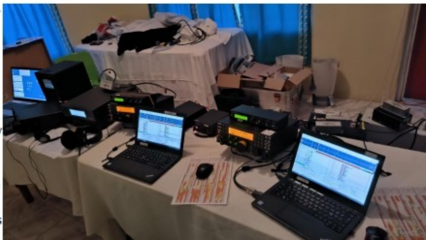
from left: FT-DX10 with EB1200, K3 with Expert 1k3; K3 w/o PA
