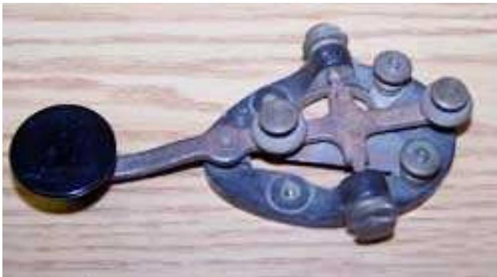
I used about a quart of Evapo-Rust in the test and it worked very well. It removed the rust from the key's steel arm in two days. I did several items with equal success. I went back to the Evapo-Rust website to research the product a little further. The process this product uses to remove rust is called chelation. The chelation agent combines with the iron oxide and kind of holds it in suspension. The result is a de-rusted object.
