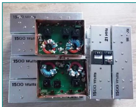
Perfo Box 1500 bandpass filters and Four-square relay switch units by RA6LBS
